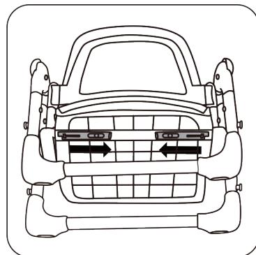
3. Ensure the catches on the bottom of the seat click in place.
