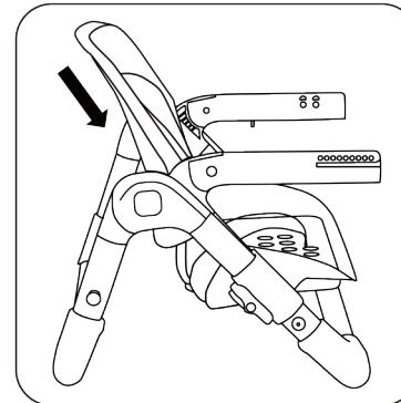
5. Align the sides of the backrest with the slots in the armrests joints and push down until they lock in place.
